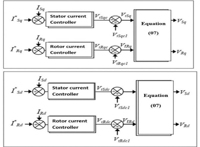
Fig. 2 Decoupling and regulation of the currents
