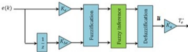
Fig. 4 Internal structure of the FLC
