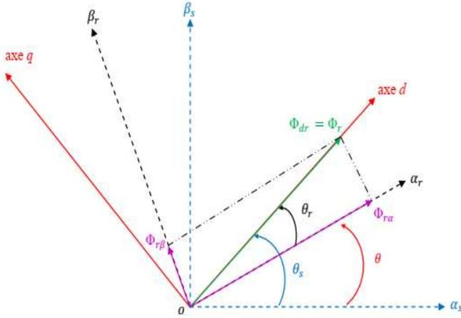
Fig. 1 Rotor field orientation on the d-axis
