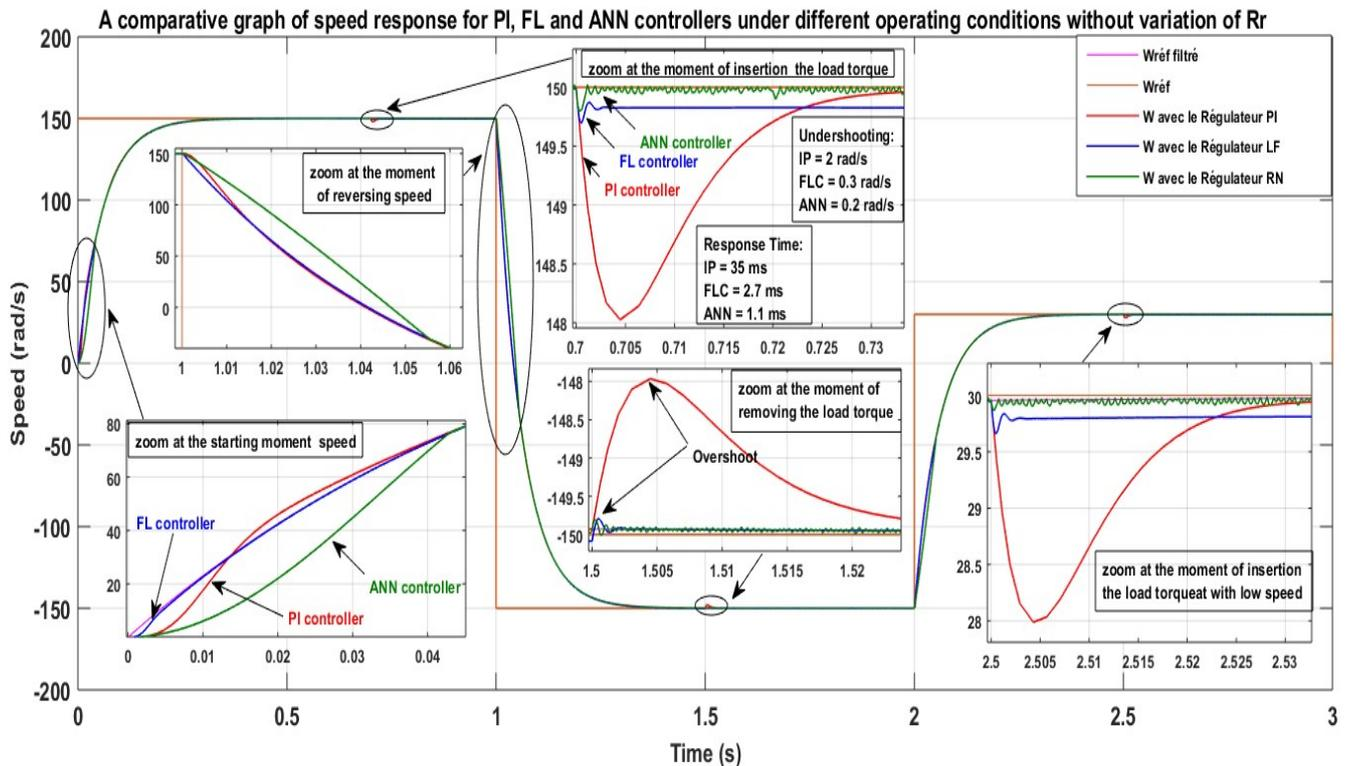
Fig.6 Simulation results of speed variation
